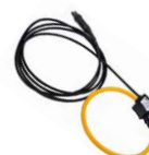
4 x F-3A flex- ible clamp (Ø=120 mm) 3 kA
