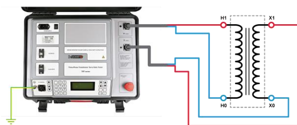
Connecting TRT to a single-phase transformer
