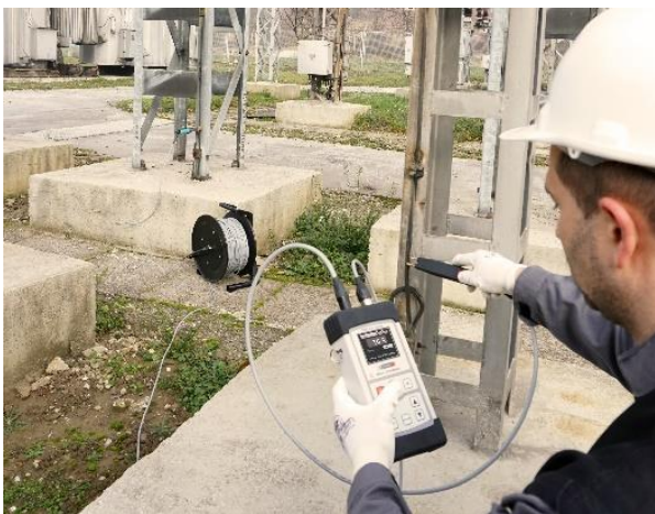
Ground grid continuity testing with RMO-EH
