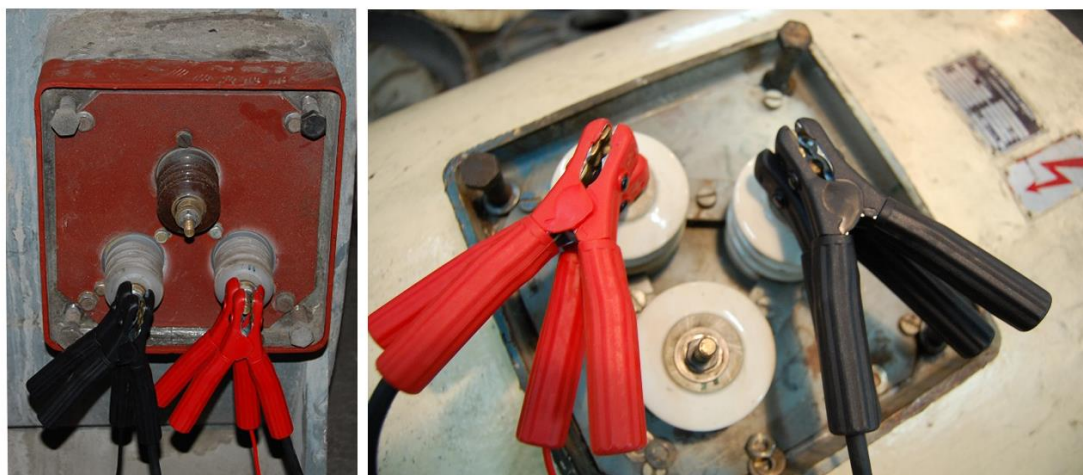
Figure 3 Connection for measuring the stator winding resistance of an asynchronous motor
